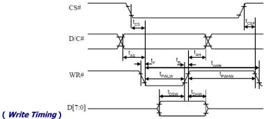
3.3.2.2 80XX-Series MPU Parallel Interface with Internal Charge Pump
